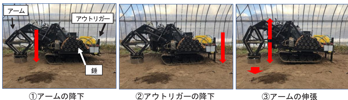
Fig.5 Procedure for pushing the insert part into the soil using outriggers
